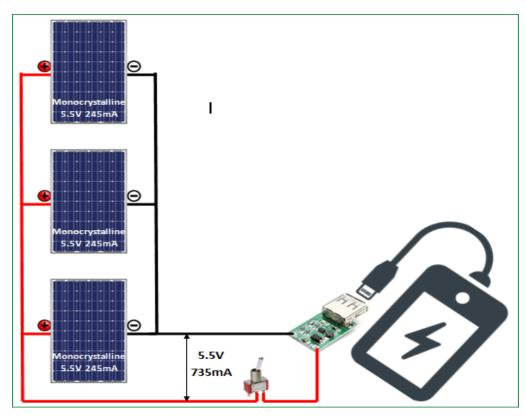
As shown in the above wiring diagram simply solder the solar panel in parallel and connect them to a boost converter module through a switch. Now simply use any power cable and connect it to the USB pin of the module and the other end to your Mobile phone. When there is proper radiation the phone will start to get charge.
